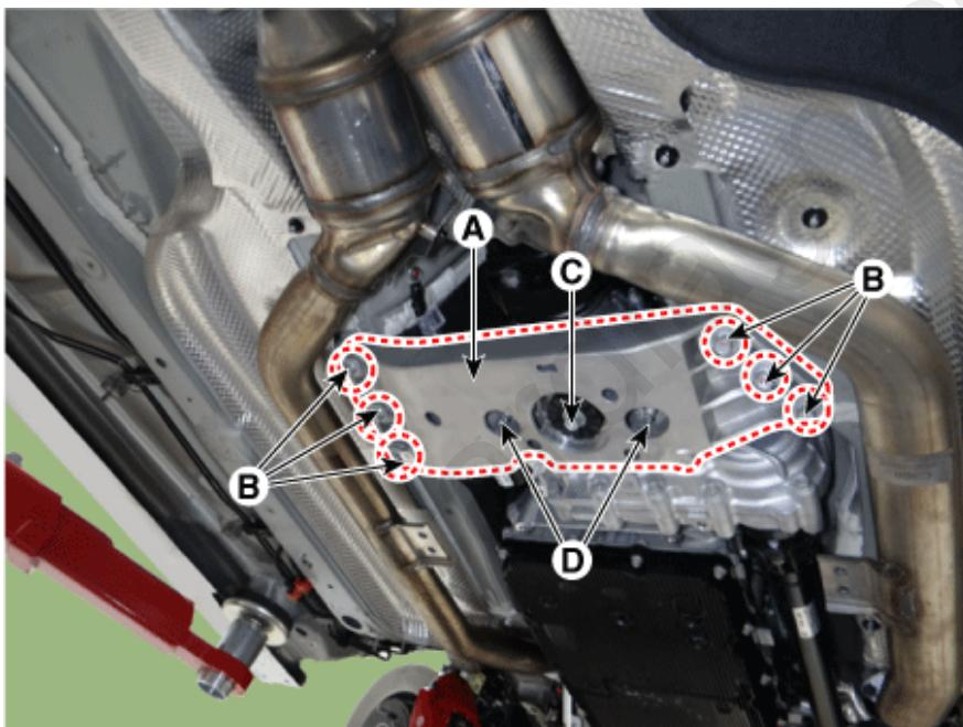
5. Remove the transmission cross member bracket (A).
