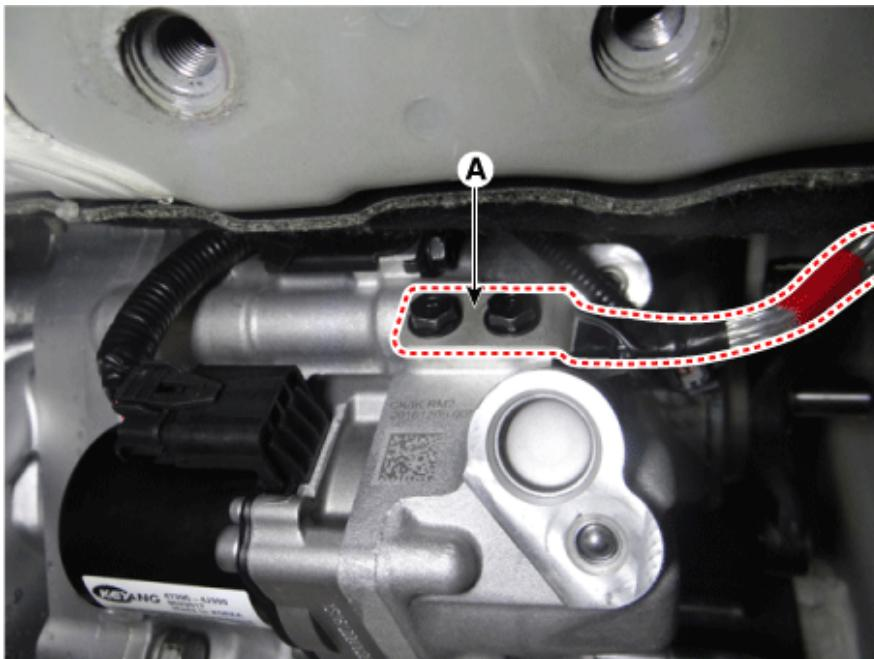
11. Remove the transfer wire ring (A).
