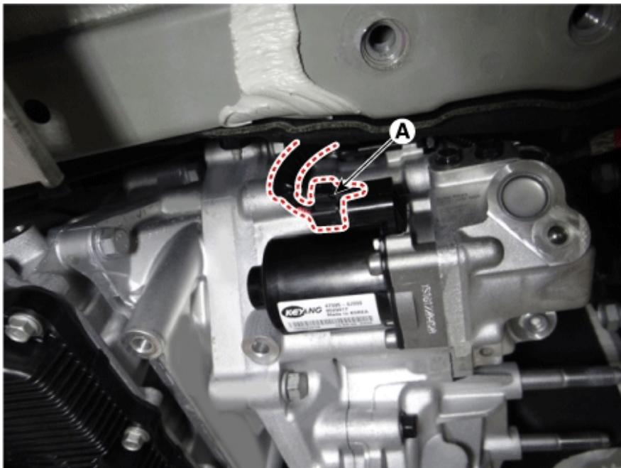
9. Disconnect the pressure sensor connector (A).
