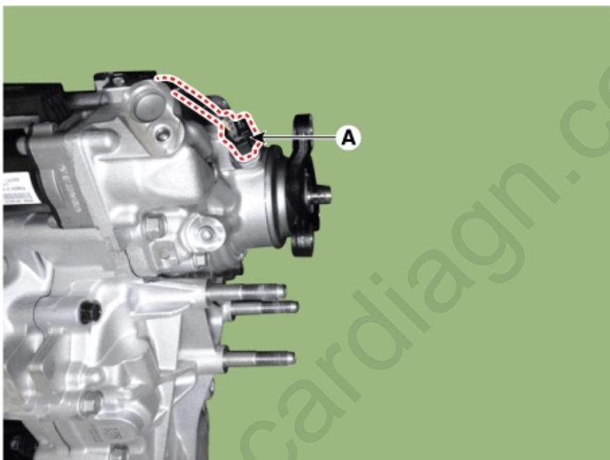
10. Loosen the bolts and then bracket (A).
